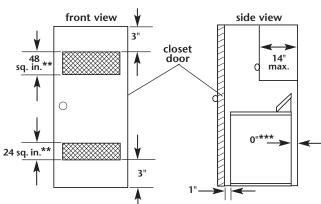
\*\* Minimum top and bottom air openings for closet door. \*\*\* External exhaust elbow requires additional space.
